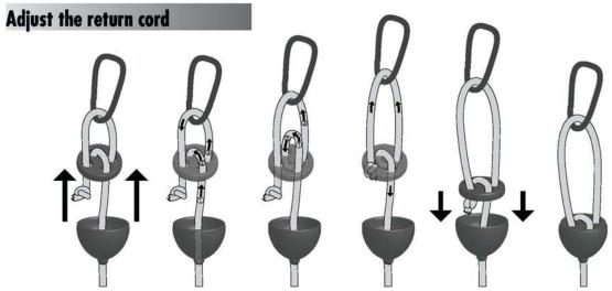
To adjust the tension of the return cord, simply adjust the length of the loop as per the above instruction. The larger loop you have fixed, the more tension you can get.
