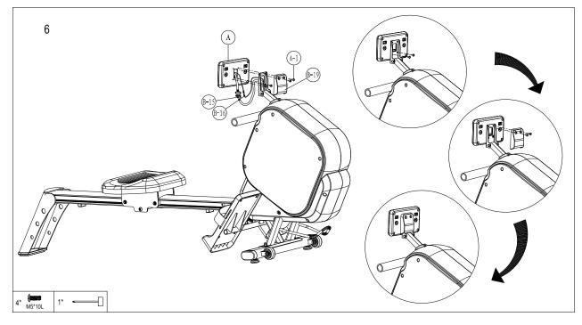
Steps 6 Plug the Adaptor (M) into the DC hole (B-14) to start the computer
