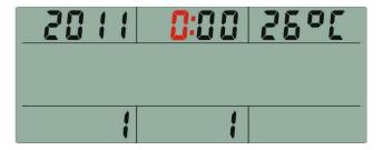
After 4 minutes without rowing, console will enter into power saving mode and display only clock, calendar and room temperature.
