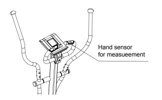
You can measure your pulse with the two hand sensor on the handle. >> Place both hands on the hand sensor on the handle as you exercise and wait briefly for the pulse to be displayed.
