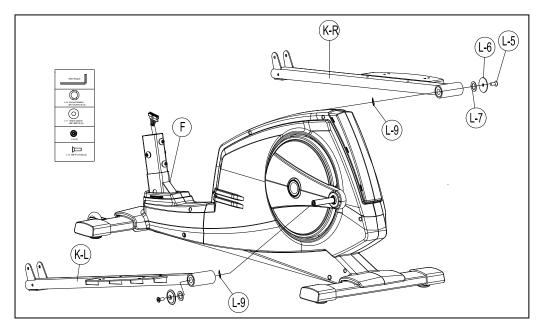
1. Assemble the R/L pedal arm (K-L, K-R) to the cross disc (F-16) by wave washer (L-9) ,flat washer (L-7) , gasket (L-6), and allen bolt (L-5).
