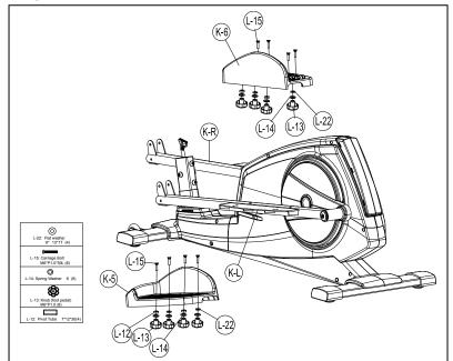
1. Put R/L pedal(K-5, K-6) onto the pedal arm (K-L/R) and tighten it, using 4 knob (L-13), flat washers (L-22), spring washer (L-14), sleeve (L-12) and bolts(L-15) in each side
