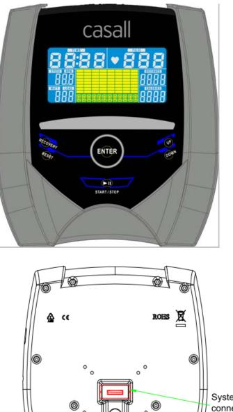
System plug connection socket
