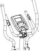
Hand sensor for pulse measurement You can measure your pulse with the two hand sensor on the handle.
