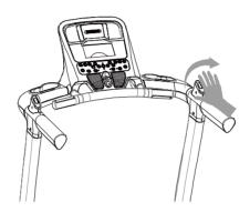
2. Wave your left hand approximately 6 cm above the motion sensor on the left handle bar to decrease the speed. The sensor will sound one short BEEP per scan and decrease speed by 0.1 km/ mph. Holding your left hand approximately 6 cm above the left sensor results in the sensor repeatedly sounding consecutive BEEPs and decreasing speed quickly by 0.1KM/H per second.
