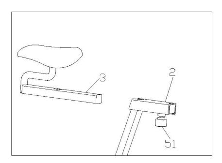
Insert the seat bracket (3) into seat post (2), 10 position can be available as per use's requirement. The seat can be slide horizontally following the arrow, then rocked strongly by the adjustable knob (51).
