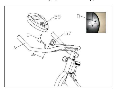
Prevent the sensor cable to touch the flywheel while the handlebar (6) is in the lowest position, Pull out the upper wire harness (56) from the hole
