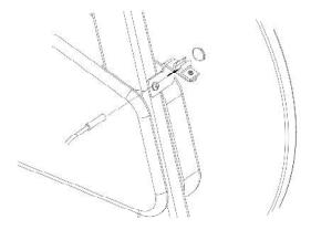
Adjust the position of sensor, ensure the distance between sensor's end and magnet is 5~8 mm.
